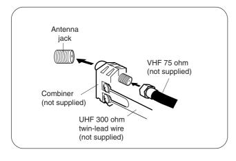
Connect the VHF 75 ohm cable and UHF 300 ohm twin-lead wire to the combiner (not supplied). Attach the combiner to the antenna jack.
